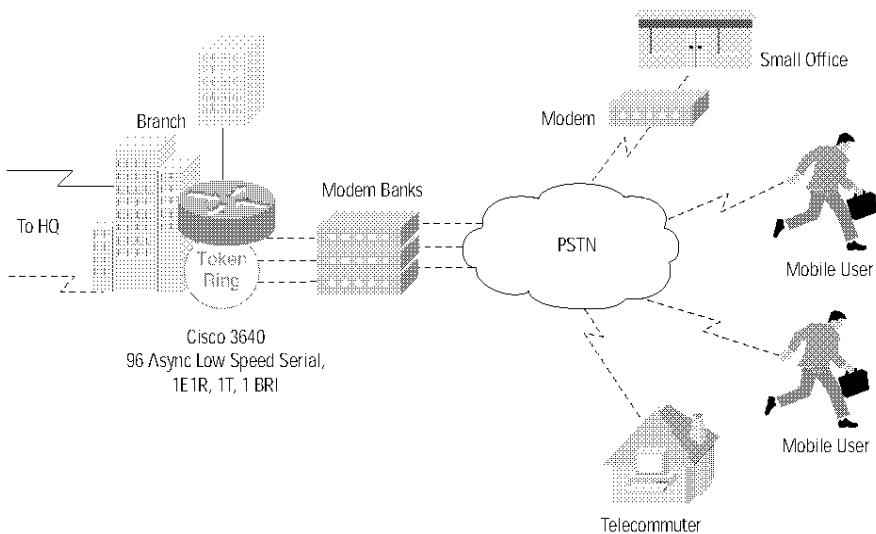
The Cisco 3600 high-density access server solution provides up to 96 asynchronous connections per chassis, delivering high performance at a competitive price per port.
