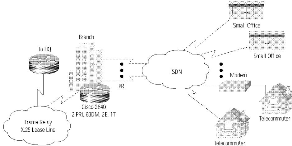
With proven performance and robust Cisco IOS WAN optimization features, a Cisco 3600 ISDN access server with integrated digital modems delivers full wire-speed performance under maximum call loads.
