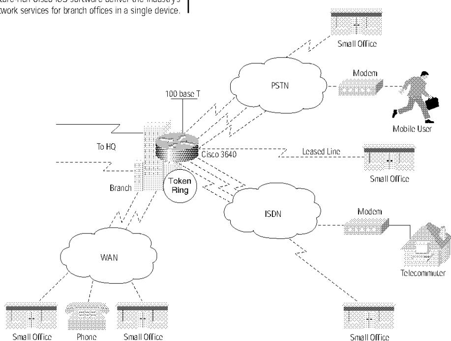
For very high-density ISDN access requirements in distributed points of presence (POPs), the Cisco 3600 server delivers the performance and robust software features that enterprises and service providers alike need in remotely managed access systems.
